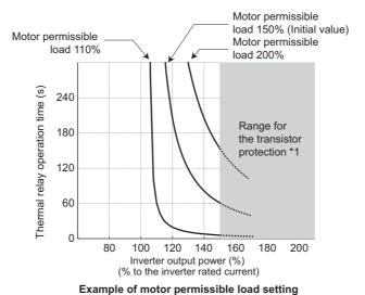
\*1 Depending on the settings of **Pr.607** and **Pr.608**, this thermal protection may not be provided as set, as an inverter overload trip (electronic thermal relay function) (E.THT) may be activated before the thermal protection.
