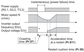
\* The output shut off timing differs according to the load condition.
