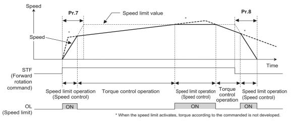
• At the STF signal ON, the speed limit value is raised in accordance with the setting of Pr.7.
