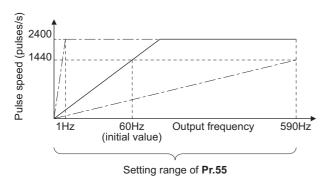
• Enter the full-scale value of the meter corresponding to a voltage of 10 VDC output via terminal AM. Enter the current value (for example, 60 Hz or 120 Hz) at full scale of the meter (10 VDC voltmeter) installed between terminal AM and terminal 5. Output voltage is proportional to the frequency. (The maximum output voltage is 10 VDC.)
