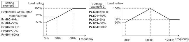
• When setting **Pr.600**, **Pr.602**, **Pr.604** (**Pr.692**, **Pr.694**, **Pr.696**) to the same frequency, the following graph's upper level is applied.
