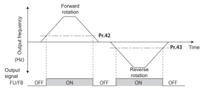
• To use each signal, set the corresponding number selected from the following table in any parameter from **Pr.190 to Pr.196 (Output terminal function selection)** to assign the function to an output terminal.
