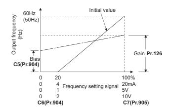
· There are three methods to adjust the bias/gain frequency setting voltage (current).
