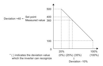
· The display of the following parameters is changed according to the C42 (Pr.934) and C44 (Pr.935) settings.
