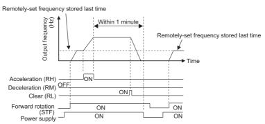
• When the remotely-set frequency is cleared by turning ON the clear (RL) signal after turning OFF (ON) both the RH and RM signals, the inverter operates at the frequency in the remotely-set frequency cleared state if power is reapplied before one minute has elapsed since turning OFF (ON) both the RH and RM signals.
