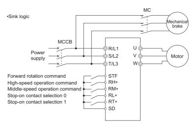
\* The input terminal used differs according to the Pr.180 to Pr.189 settings.
