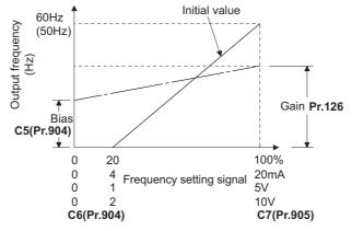
Other adjustment methods for the frequency setting current gain are the following: adjustment by applying a current through terminals 4 and 5, and adjustment using a specified point without applying a current through terminals 4 and 5. (Refer to page 318.)
