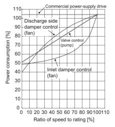
• The estimated input power (kW) for the commercial power supply operation is calculated from the motor capacity set in **Pr.893**, the setting of **Pr.892 Load factor**, and the rate of power consumption using the following formula.
