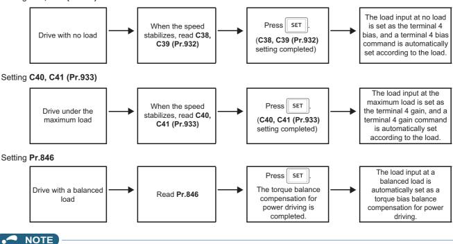
• To perform a torque bias operation after the automatic setting is completed, set Pr.840 to "1" or "2".
