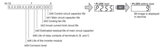
• When the parts have reached the life alarm output level, the corresponding bits of **Pr.255** turns ON. The ON/OFF state of the bits can be checked with **Pr.255**. The following table shows examples.
