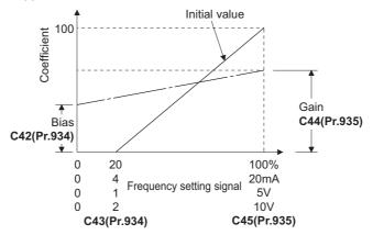
There are three methods to adjust the PID display bias/gain.
