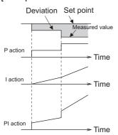
(Note) PI action is the result of P and I actions being added together.
