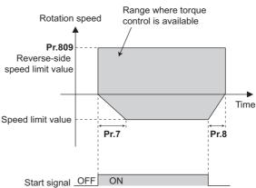
When the torque command value is negative
