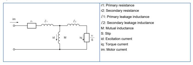
In the above diagram, currents flowing in the induction motor can be classified into a current id (excitation current) for making a magnetic flux in the motor and a current iq (torque current) for causing the motor to develop torque.
