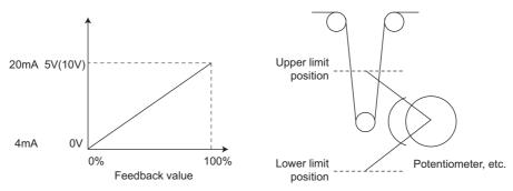
(Example) To execute control at the dancer center position using a 0 to 7 V potentiometer
