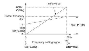
• Other adjustment methods for the frequency setting voltage gain are the following: adjustment by applying a voltage directly across terminals 2 and 5, and adjustment using a specified point without applying a voltage across terminals 2 and 5. (Refer to page 318.)
