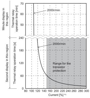
Protective function activated area: the area right of the characteristic curve Normal operation area: the area left of the characteristic curve
