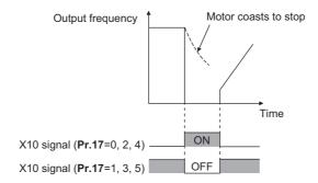
· Relationship between Pr.17 and the Inverter run enable signal of each option unit
