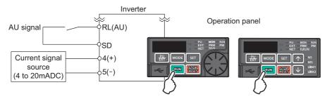
The following shows the procedure to operate at 60 Hz.
