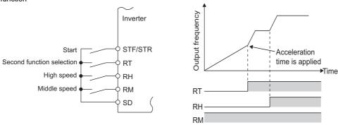
• When the RT signal is ON, second functions are selected. The following table shows the functions which can be changed to the second function.
