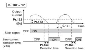
\* When the output is restored to the Pr.152 level, the Y13
