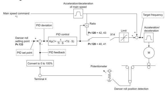
1 The main speed can be selected in all operation modes, External (analog voltage input, multi-speed), PU (digital frequency setting) and Communication.
