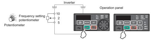
The following shows the procedure to operate at 60 Hz.
