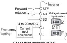
Connection diagram using terminal 4 (4 to 20mADC)
