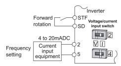
Connection diagram using terminal 2 (4 to 20mADC)
