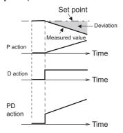
(Note) PD action is the result of P and D actions being added together.
