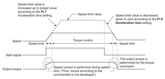
• If the setting value of **Pr.7 and Pr.8** is "0", turning OFF the start signal enables speed control, and the output torque is controlled by the torque limit value.
