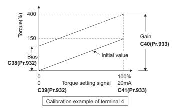
There are three methods to adjust the bias/gain for torque setting current (voltage).
