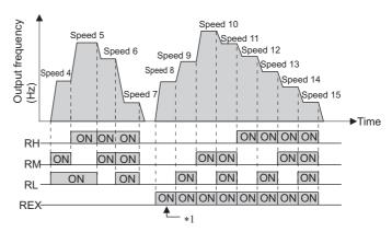
When the RH, RM and RL signals are OFF and the REX signal is ON while "9999" is set to Pr.232 Multi-speed setting (speed 8), the inverter operates at the frequency set in Pr.6.
