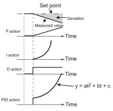
(Note) PID action is the result of all P, I and D actions being added together.
